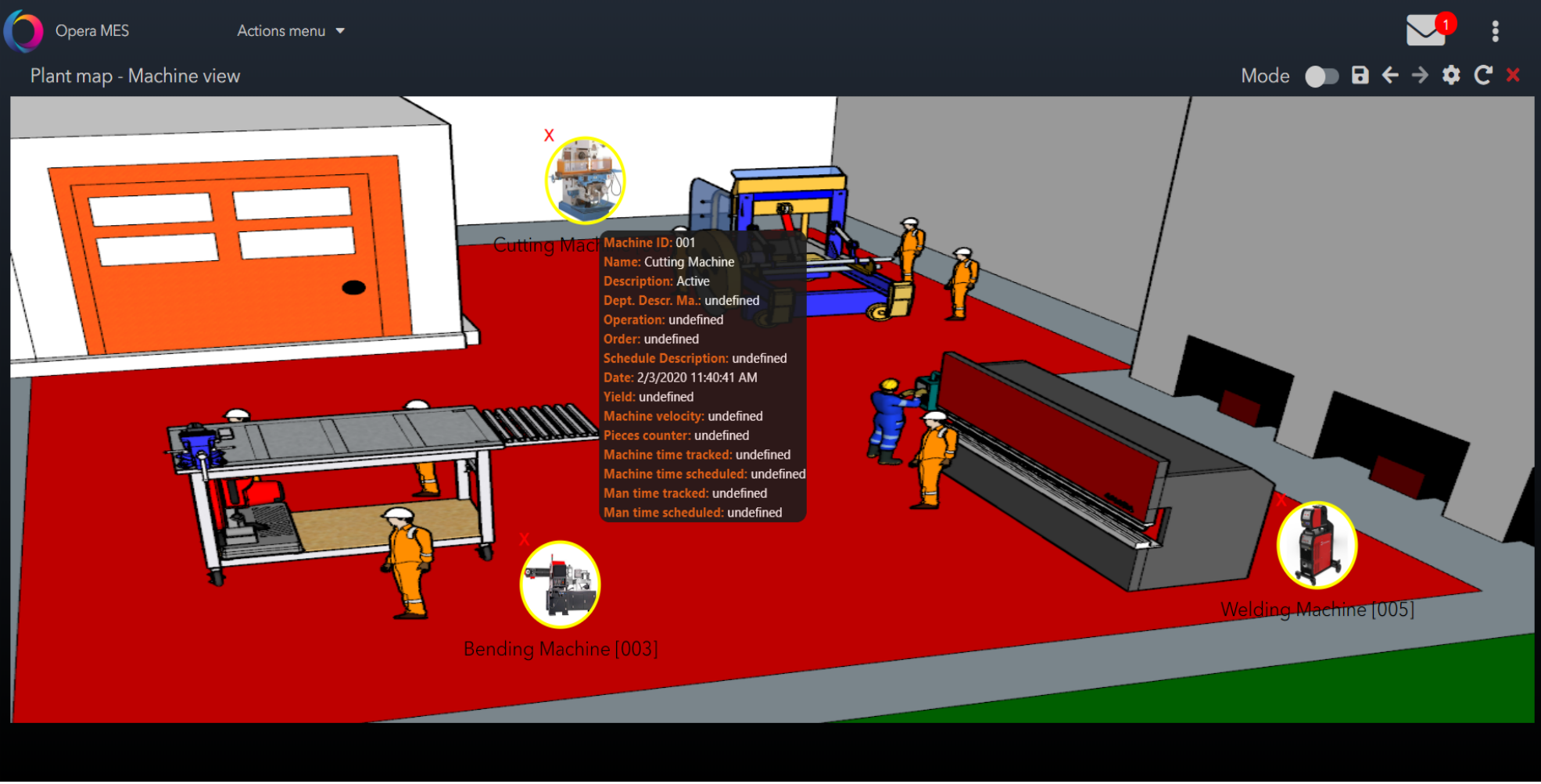
Map of a specific department with production progress data for each machine in real time.
